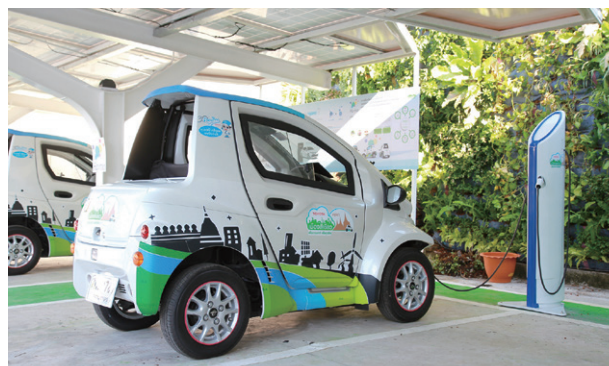
A Ha:mo vehicle being charged with carbon-free renewable electricity generated from solar panels installed on the roof of the parking facility
